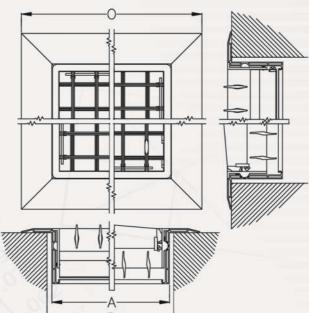
Adjustable ceiling diffusers are produced with beautiful appearance, light weight, suitable airflow, easy installation and easy cleaning features. In these types of diffusers, merely the main frame is connected to duct system or ceiling via bolt and grilles or grids are easily installed or disconnected without any special tool.
