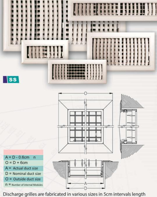
Discharge grilles are fabricated in various sizes in 5cm intervals length and height. Minimum size of discharge grilles is 10cm height and 15cm length.
