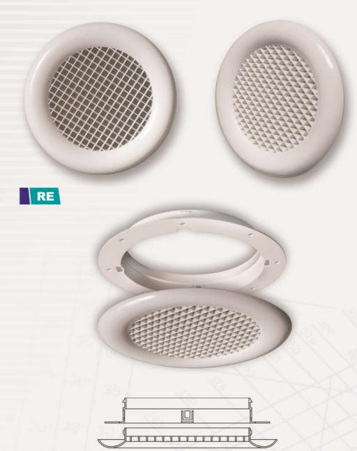
ARYAN ARVIN plastic round grilles have beautiful appearance, light weight, suitable airflow, easy installation and easy cleaning capabilities. These grilles have an adaptor that is connected to duct or ceiling and grilles are easily installed or disconnected from this adaptor. These grilles are produced in 10cm, 15cm, 20cm, 25cm and 30cm diameters. These grilles are fabricated from industrial ABS.
